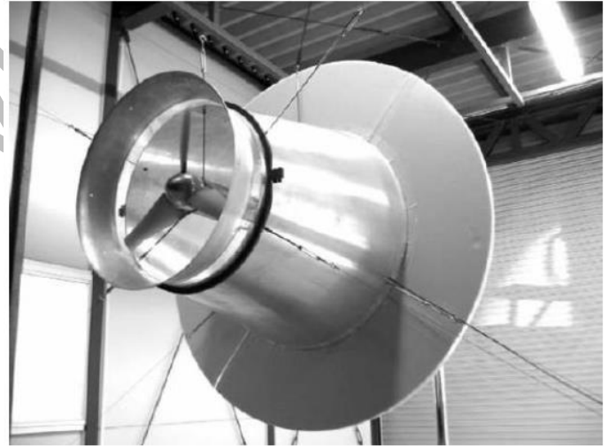
Figure 1: Schematic of a conventional horizontal axis wind turbine with a flanged diffuser [7]
