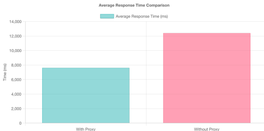
Figure 2: Response times comparison - Naive Append without proxy vs Context Pruning with proxy
