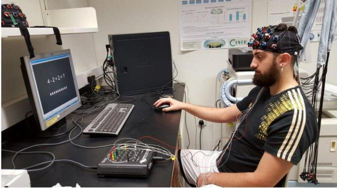
**Figure 1.** The setup of multi-modal fNIRS-EEG experiment for subject performing arithmetic task.
