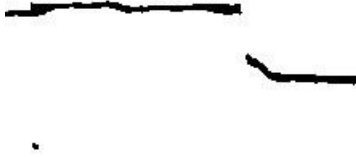
311 Fig. 18: Crack detection after noise reduction
