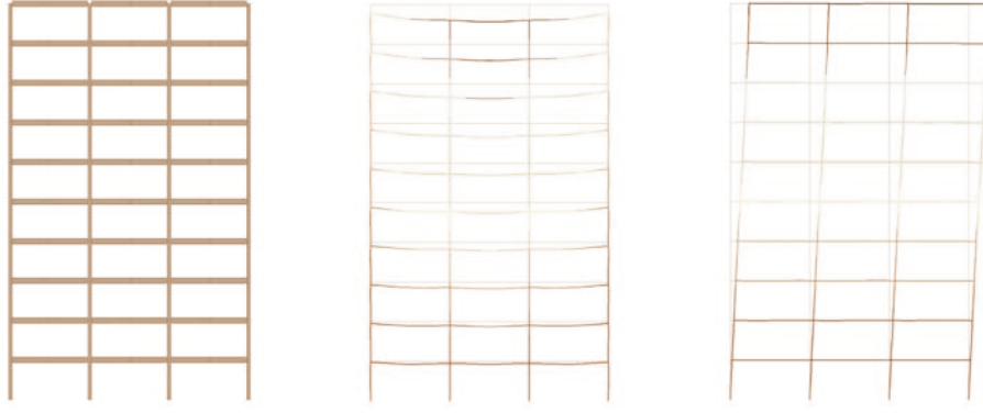
FIGURE 4.1. Example 1 and its gravitational (middle panel) and lateral deflections (right panel).
