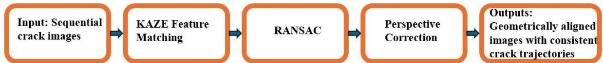
Fig. 2.4: Full alignment pipeline from keypoint extraction to geometric correction
