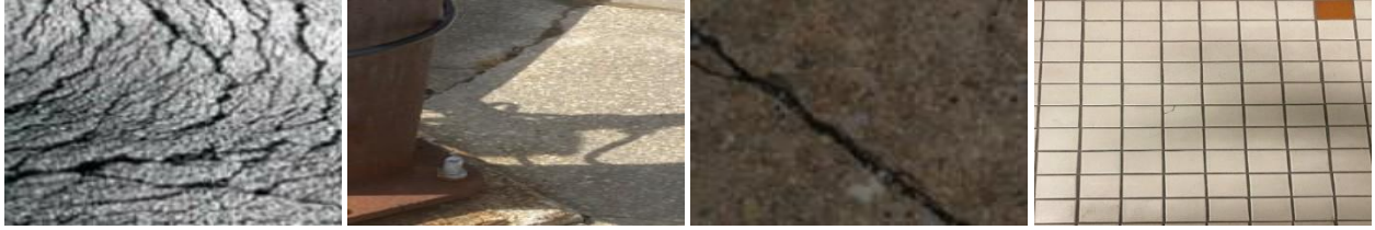
(a) Non-planar surfaces (b) Occlusion or low visual salience (c) Poor image quality (d) Short or textureless cracks
