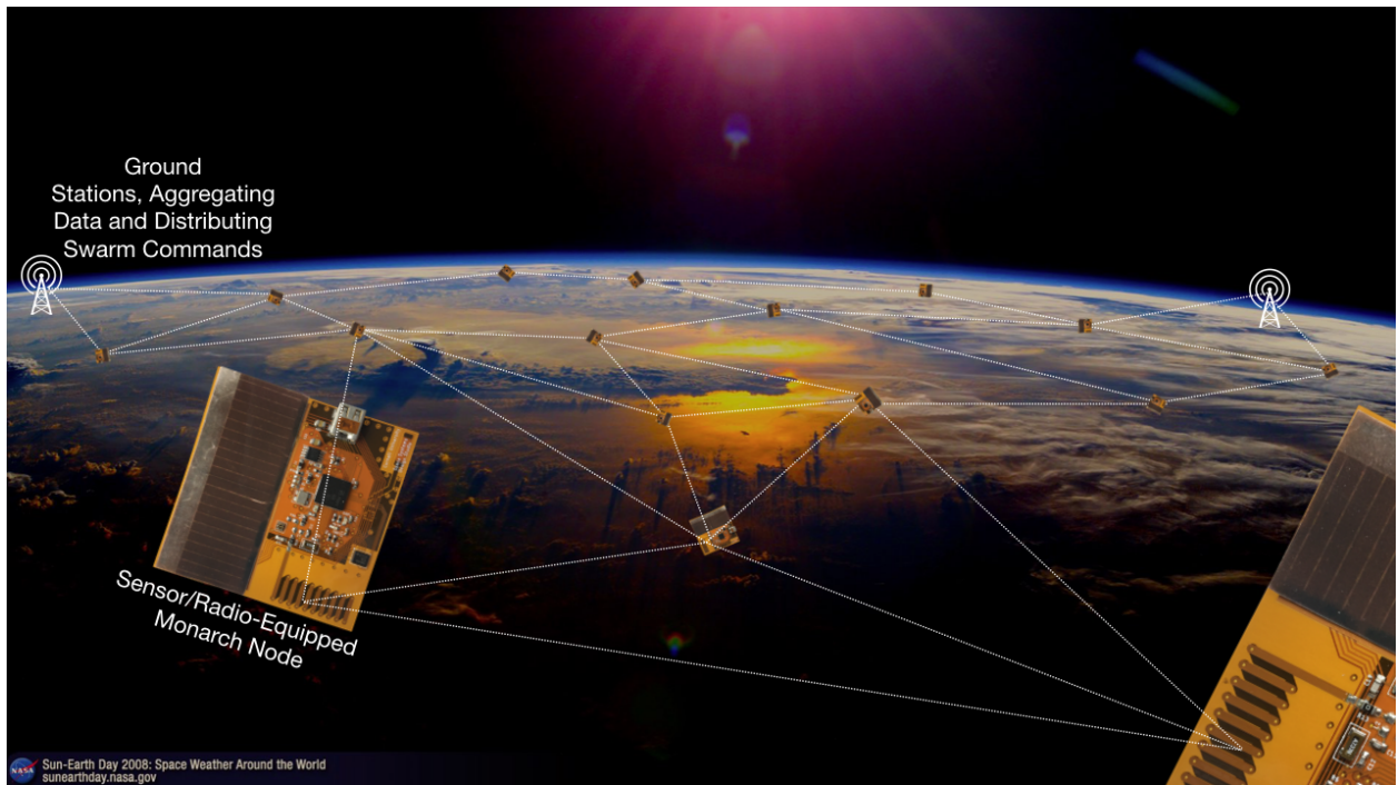
Fig. 4 Artistic representation of a swarm of networked Monarchs performing a distributed in-situ sensing mission in low-Earth orbit.
