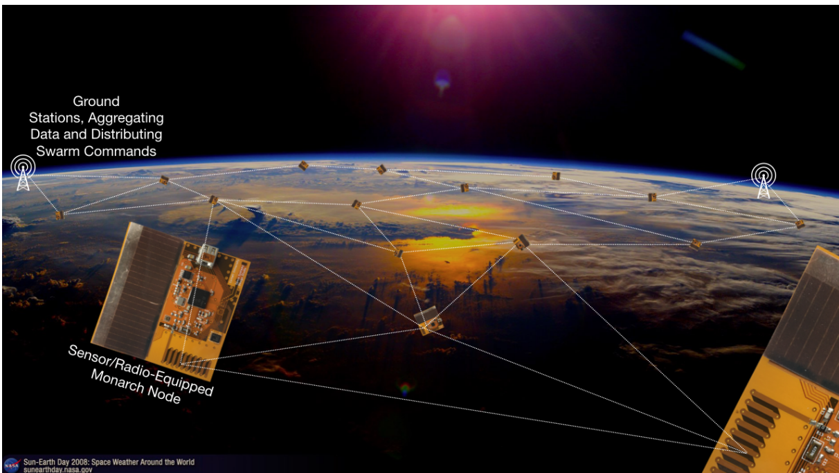
Figure 3: Artistic representation of a swarm of networked Monarchs performing a distributed in-situ sensing mission in low-Earth orbit.
