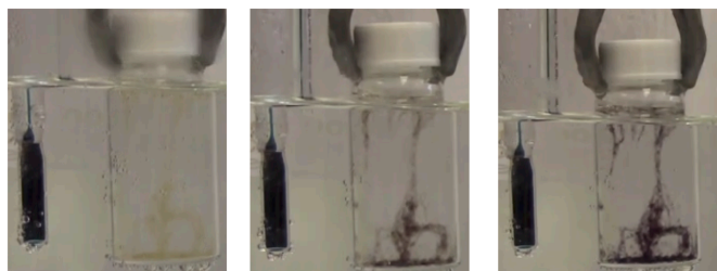
Figure 6. Images from a video recording of a fiber formation reaction (0.25 mM HAuCl 4 and 5.6 μM lysozyme in 20 mL of water heated at 80 °C).
