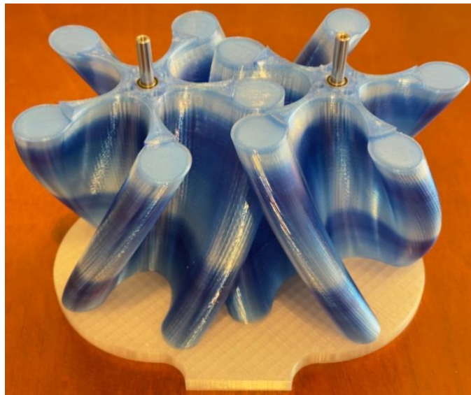
Figure 8. 3D-printed 5-lobe rotors with helix angle 72^\circ and \epsilon = 0.3
