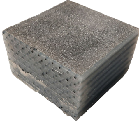
Figure 2: TPU-silicone fiber-reinforced transversely isotropic composite. Note the speckle pattern applied to the top surface to allow surface deformation measurement around the indenter, using DIC.
