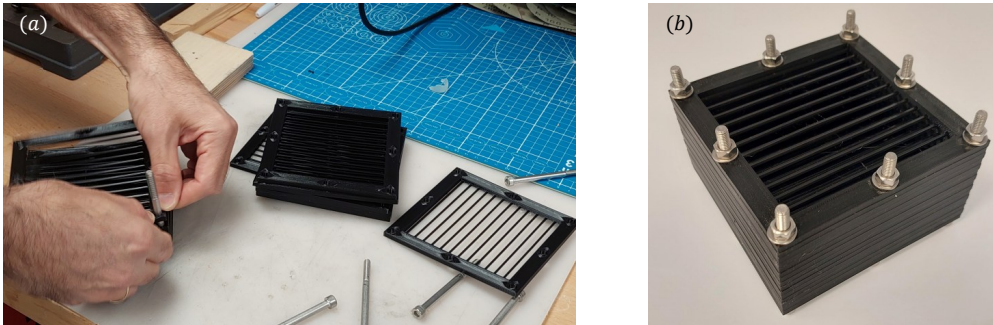
Figure S1: Mold preparation with 3D-printed TPU sheets and uniformly spaced fibers. (a) Assembling the mold, and (b) the prepared mold.
