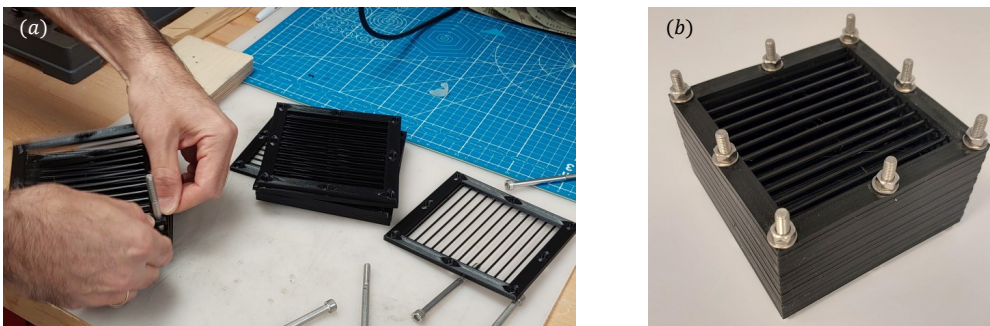
Figure A.17: Mold preparation with 3D-printed TPU sheets and uniformly spaced fibers. (a) Assembling the mold, and (b) the prepared mold.
