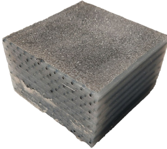
Figure 2: TPU-silicone fiber-reinforced transversely isotropic composite. Note the speckle pattern applied to the top surface to allow surface deformation measurement around the indenter, using DIC.
