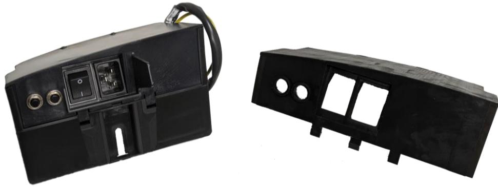
Figure 9. Left: Original assembly. Right: Printed replacement part.
