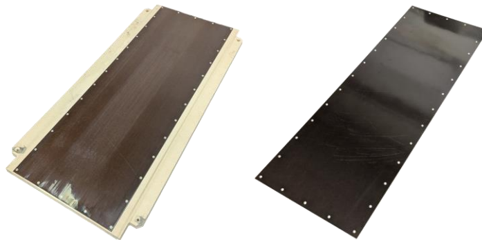
Figure 11. Left original assembly. Right: Machined replacement part.
