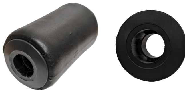
Figure 10. Left: Original assembly. Right: Printed replacement part.
