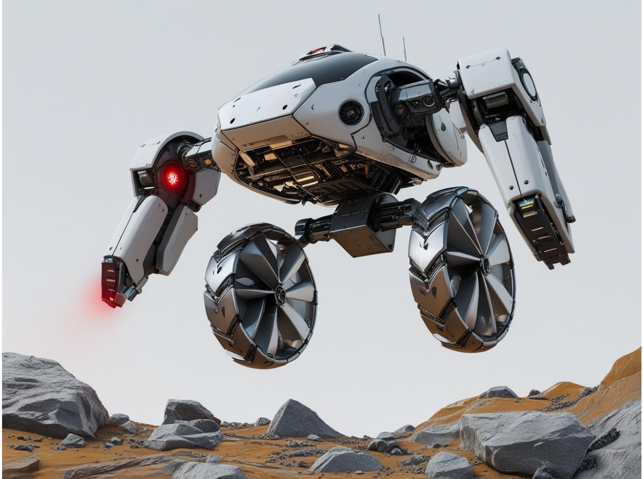
Figure 6: 3D rendering of the ASTRA prototype during its mid-air transformation. The vehicle is descending over rocky terrain as its thruster shrouds pivot and unfold to form wheels. A damaged actuator node on one of the hinges glows red, indicating the initiation of the self-healing cycle (healing demonstrated in lab conditions).
