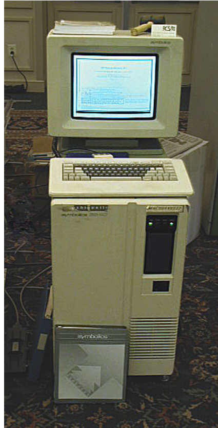
Figure 1.3: A Symbolics Lisp Machine, a specialized hardware platform designed to run expert systems which are a version of AI focusing on answering questions to challenging problems. a
