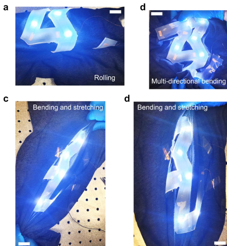
Figure S11. Application of CuLMCs as stretchable and wearable interconnects mounted on textiles under extreme conditions. (a) Rolling. (b) Multi-directional bending. (c-d) Simultaneous bending and stretching from diagonal direction and vertical direction. The luminosity is stable for all cases. Scale bar, 3cm.
