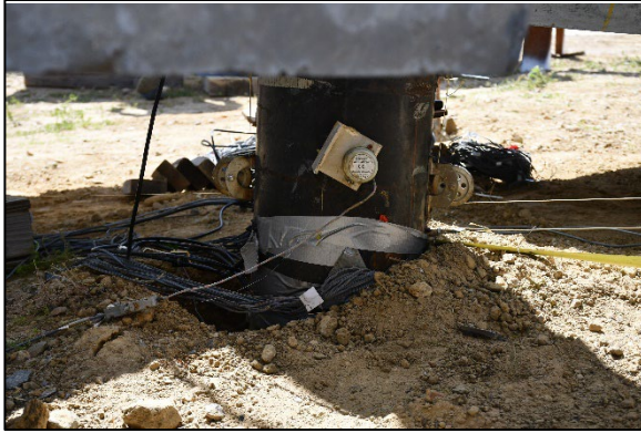
(a) Soil Gapping Field Photo at Large Amplitude Displacements
