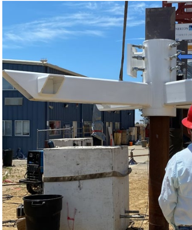
String Pot Eyebolt (x2) Installation Position Minimum 1" apart no more than 3" apart. (Closer the better)
