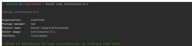
Fig. 23. A docker scan demonstrating no vulnerabilities found in the dependencies or transitive dependencies of Atlas.
