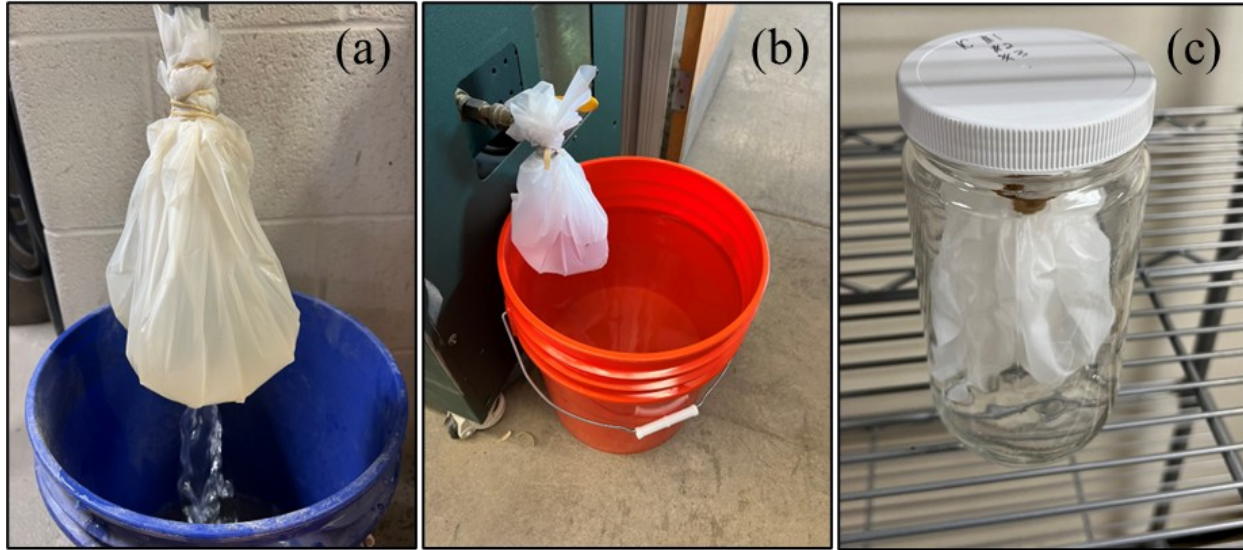
Figure 4: Sample collection from (a) HWTT, (b) MiST, and (c) sample transferred to a jar
