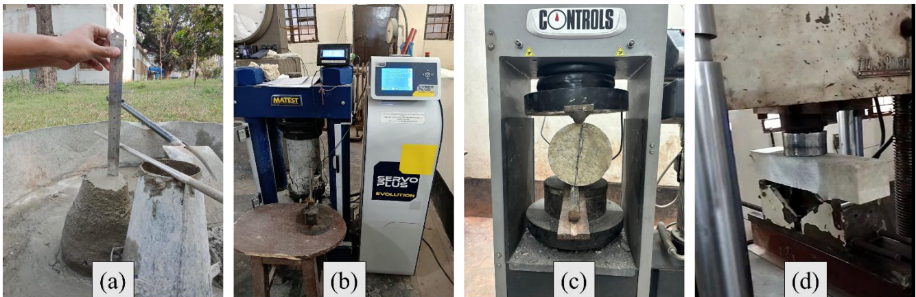
Figure 4: Rheological & Mechanical Properties Testing of Geopolymer Concrete Specimen; (a) slump, (b) compression test, (c) split tensile test, (d) flexural test.
