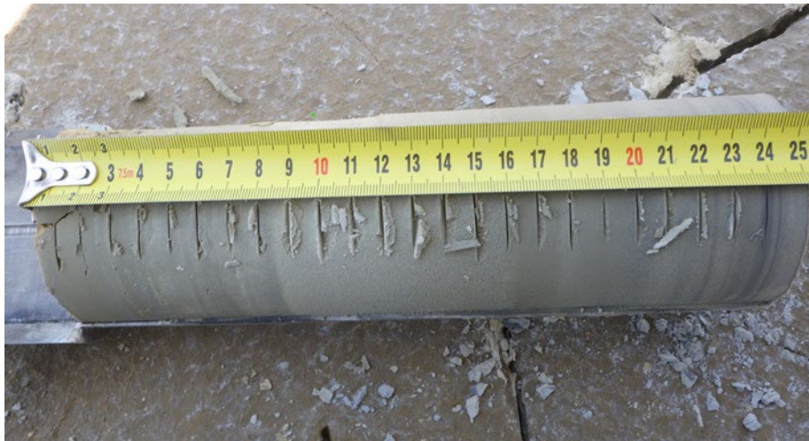
41 Fig. S4. Sample 'Spigot @100' with marks at 1 cm intervals prior to being sliced.
