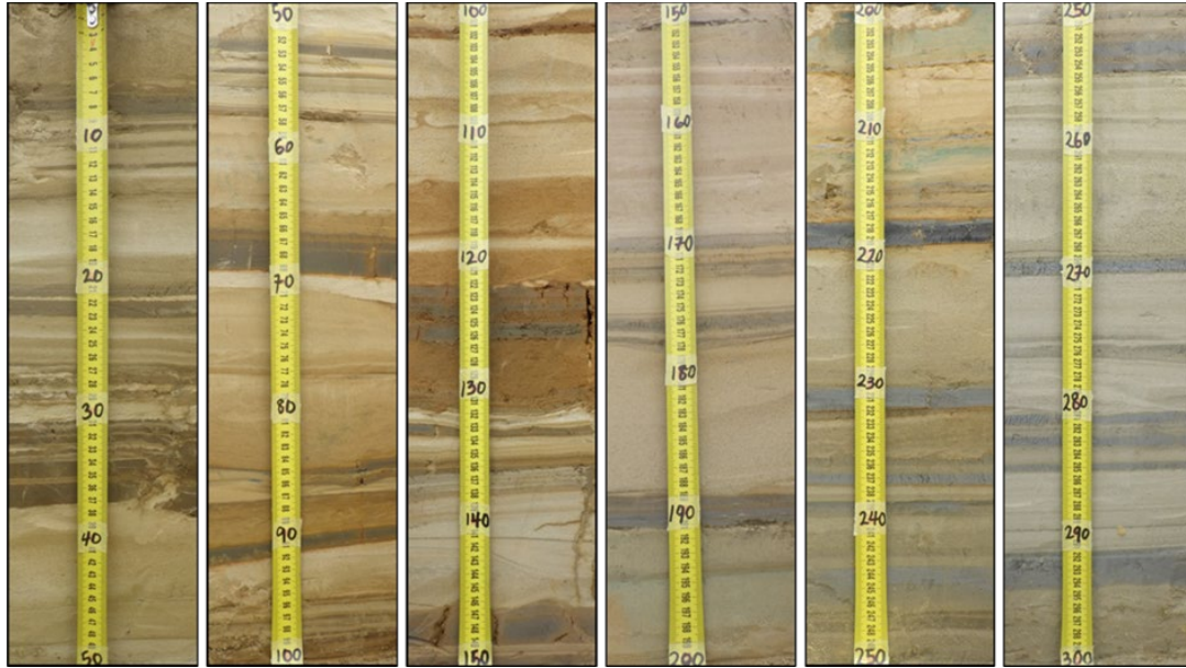
107 108 Fig. 3. The 3 m deep profile exposed at the Remine TSF. The measuring tape is graduated in centimetres.
