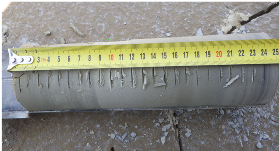
143 Fig. 4. Sample 'Spigot @100' with marks at 1 cm intervals prior to being sliced.
