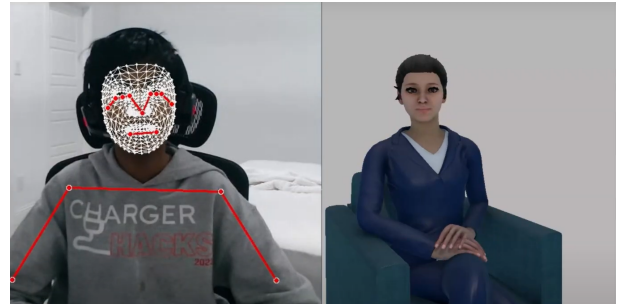
Figure 2: Sample frame from an interaction between an ECA and a user. The ECA maintains a neutral listening position as the user speaks. Mediapipe tracks real-time visual features.
