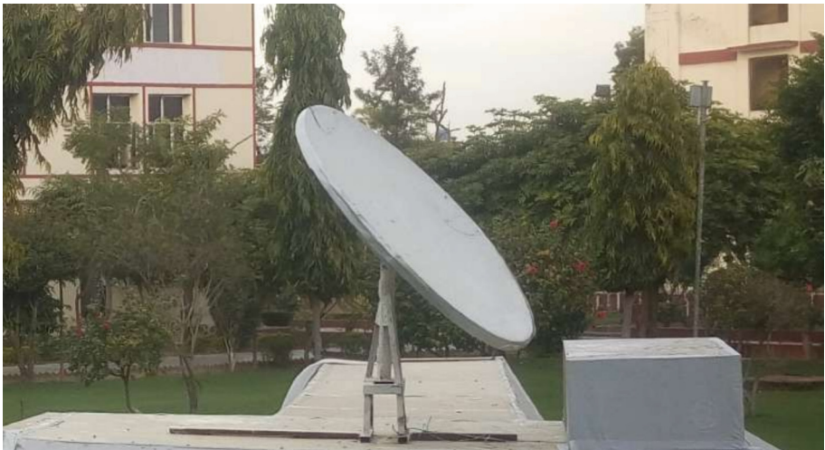
Fig. 20. Communication acoustic dish with custom welded tripod demonstrator – module 1729
