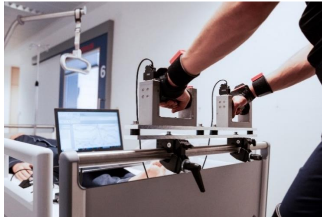
Fig. 3. Mounting of force handles on the hospital bed. The handles comprised a plastic grip, which was connected on both sides to three-dimensionally measuring piezoelectric force sensors housed in an aluminum casing containing the amplifier electronics.
