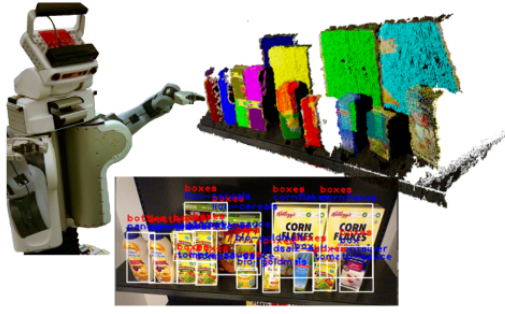
Fig. 1: Retail environment featuring the robotic agent and identified objects within a sample scene.
