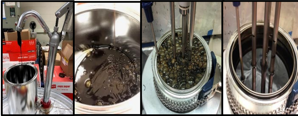
Figure 3. Processing Stages of Guayule Resin from Initial Storage to Heat Treatment
