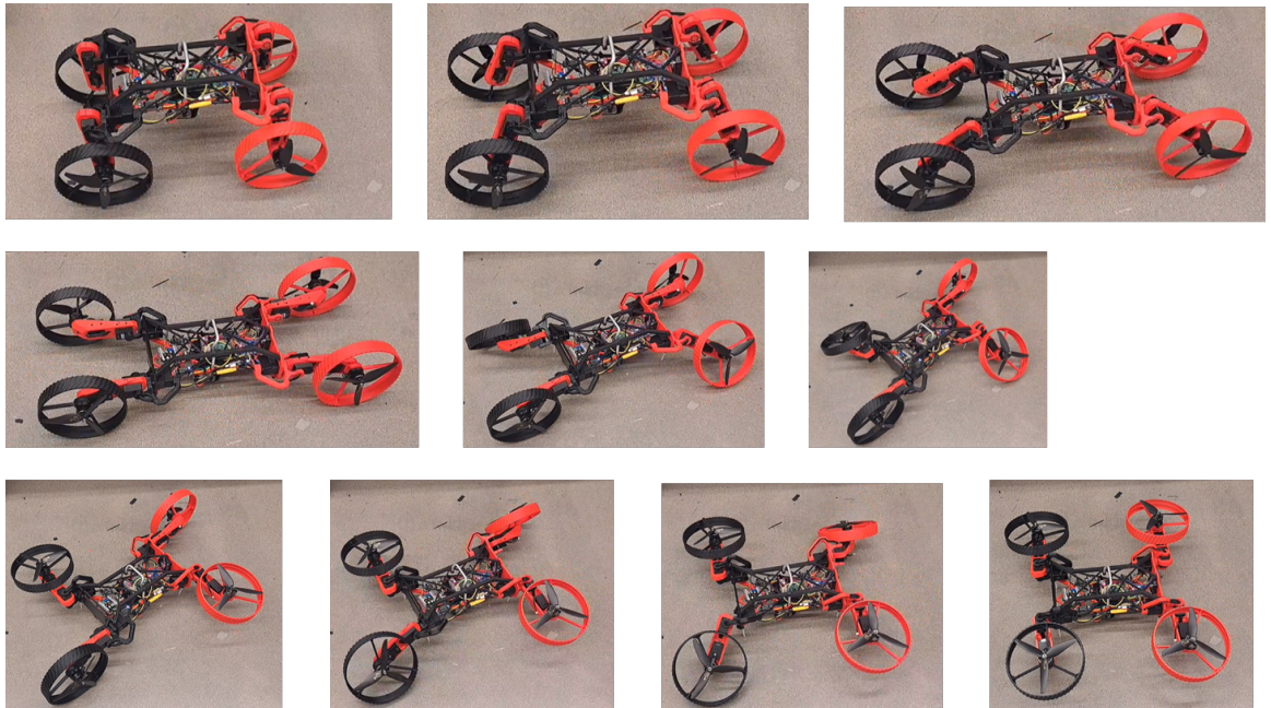
Figure 4.3: Shows M4 prototype executing morphing from crawling configuration to flight configuration.
