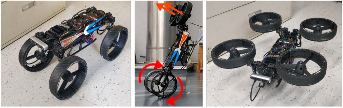
Figure 1.3: The M4 robot in various morphing configurations: rover, segway, drone [30].
