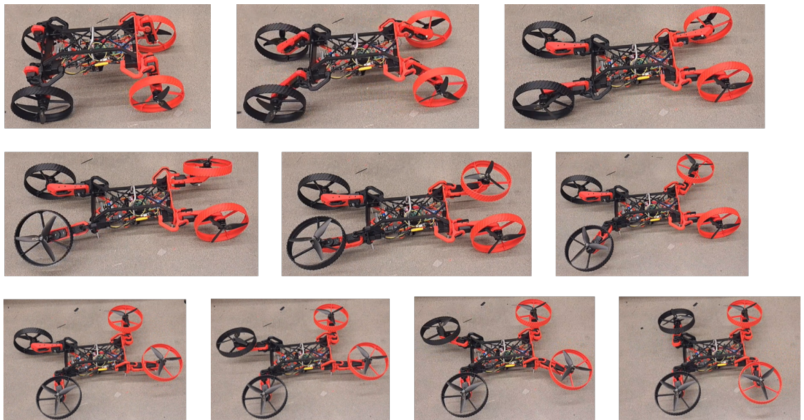
Figure 4.4: Shows M4 prototype executing a different sequence of morphing from crawling configuration to flight configuration.
