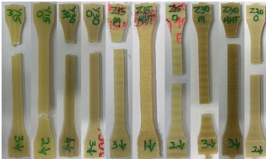
Fig 58. Comparison of fracture surfaces after the tensile test.
