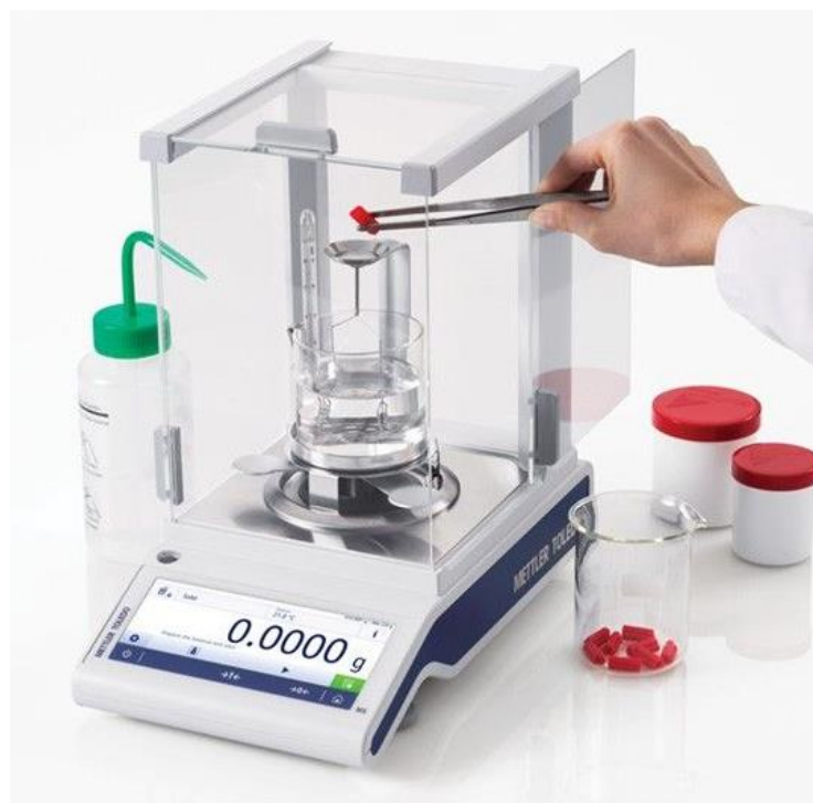
Fig 28. Density measurement using Mettler balance [29].
