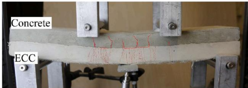
Figure 7. Crack patterns of ECC-concrete composite under flexural loading, adapted from Ref. [51].
