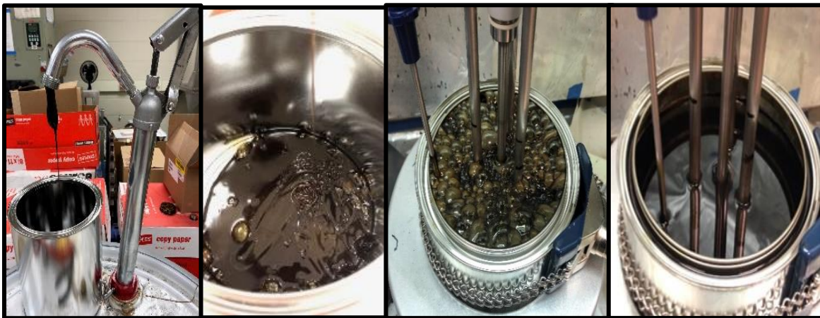
30 31 Figure 1. Sequential Stages of Guayule Resin Conditioning: (1) transfer from storage container, (2) resin in 32 raw form, (3) initiation of thermal mixing at 160^{\circ}\text{C} with moisture bubbling, and (4) post-conditioning 33 homogeneous molten resin.
