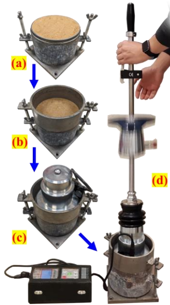
FIG. 2 LWD test on Proctor mold
