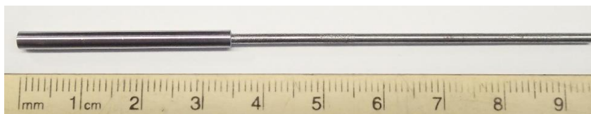
Figure 4. 1200 grit polished boiler tube steel (SA210-A1) working electrode.
