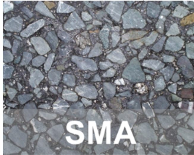
Figure 1.: Heterogeneous structure of an SMA mixture.
