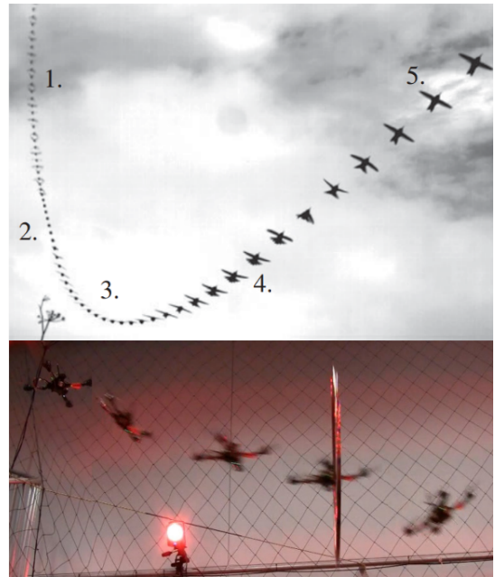
Fig. 1. (a) The five stages of an Anna’s Hummingbird dive maneuver, from [1]. (b) A quadrotor using path planning to fly through a thrown hoop, from [1].
