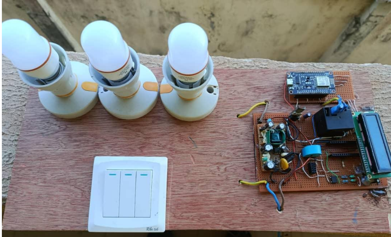
Figure 2 Smart Circuit Breaker System
