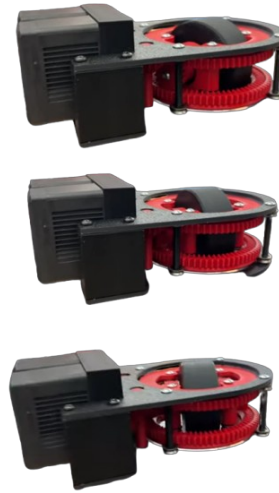
Fig. 9: Single pod movement test, where we input random positions and velocities and see how the swerve pod performs
