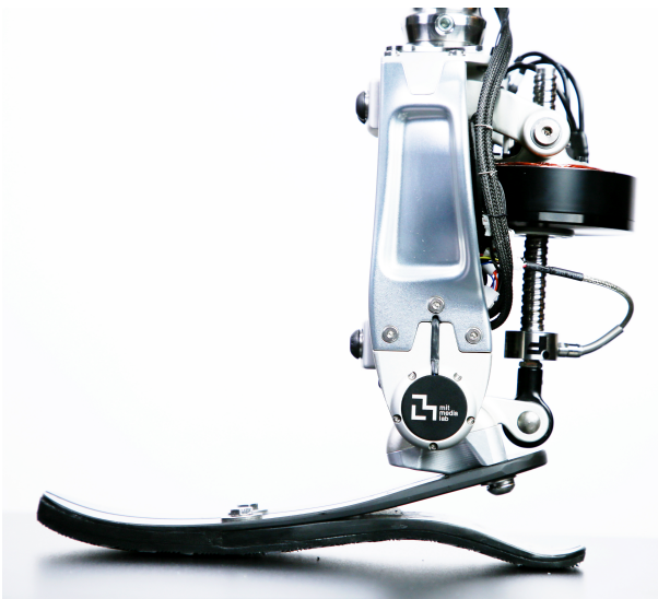
Fig. 1. The TF8 Actuator is designed to operate as either a knee or ankle actuator – shown here configured as an ankle prosthesis. Borrowed with permission from [24].
