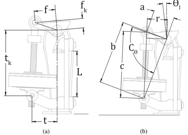
Fig. 3. (a) The actuator geometry parameters  $t$ ,  $t_k$ ,  $f$ ,  $f_k$ ,  $L$  are found through optimization. The objective was finding moment arm geometry with the most efficient configuration of the power stroke as specified by the load trajectory and actuator dynamics. (b) Parameters used for calculating instantaneous moment-arm length for control.
