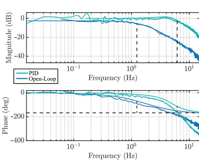
Fig. 10. Open-loop frequency response shows a damped second order system with natural frequency at 1.5 Hz and phase margin of  $-80^\circ$ . Closed-loop (PID) frequency response shows a damped second order system with natural frequency at 3.9 Hz, control bandwidth at 6.2 Hz, and phase margin of 61.5 degrees. The solid line is the estimated system response.
