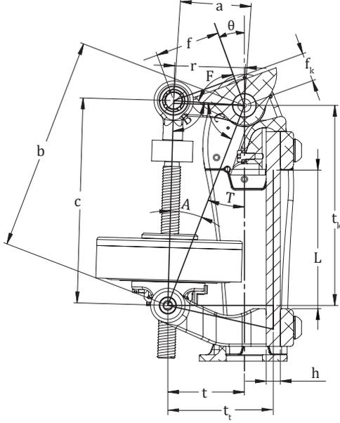
Fig. 2. Linkage geometry labels. The optimization procedure searched for the  $t, t_k, f, f_k, L$  geometry parameters. The objective was finding moment arm geometry with the most efficient configuration of the power stroke as specified by the load trajectory and actuator dynamics.
