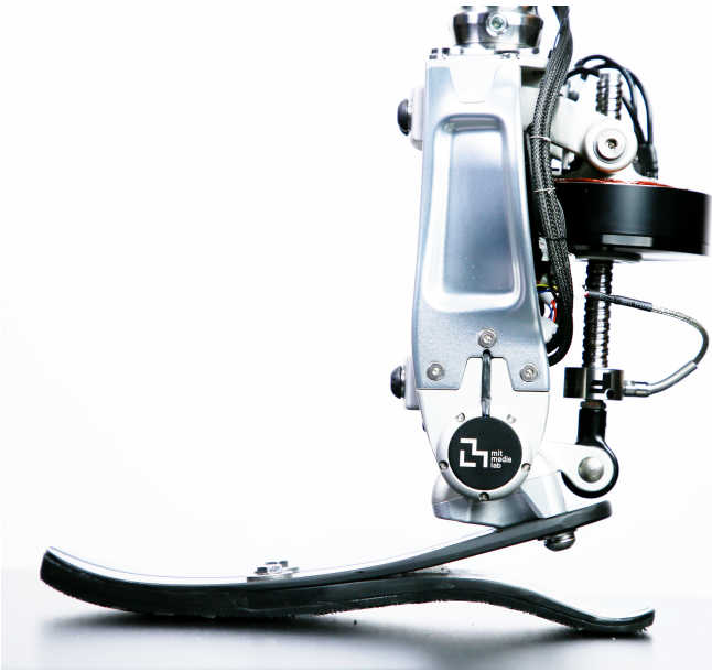
Fig. 1. The TF8 Actuator is designed to operate as either a knee or ankle powered prosthesis – shown here it is configured as an ankle prosthesis.
