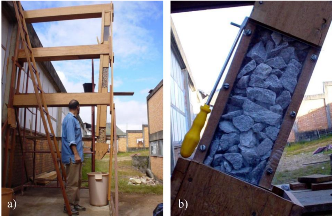
Fig. 1 a) Experimental ore pass used for testing. b) Example of granular flow obstruction due to the formation of a mechanical arc
