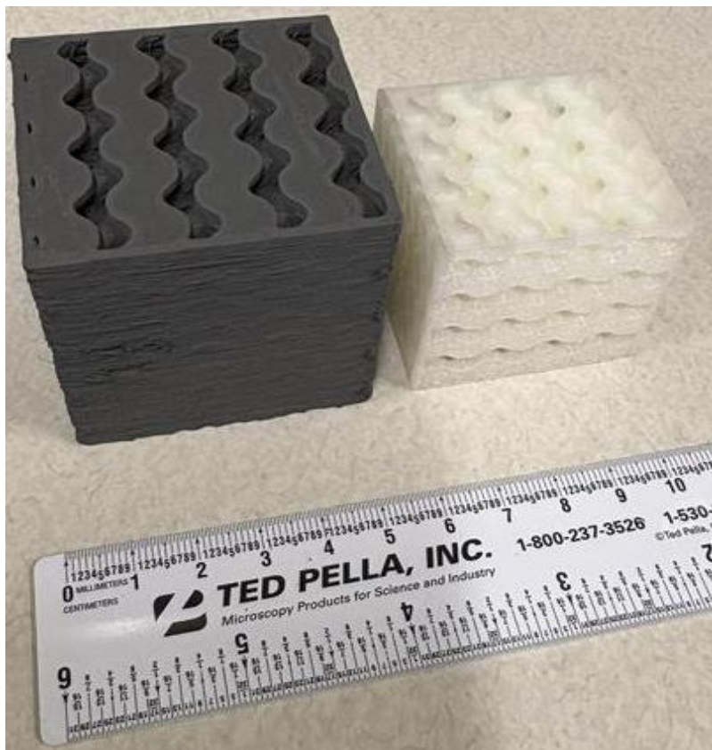
Figure 1. Gyroids of cubic edge length (left) 5 cm and (right) 4 cm printed at the Manufacturing Demonstration Facility at ORNL.
