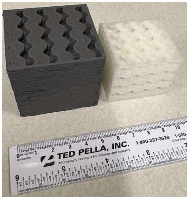
Figure 1. Gyroids of cubic edge length (left) 50 mm and (right) 40 mm printed at the Manufacturing Demonstration Facility at ORNL.
