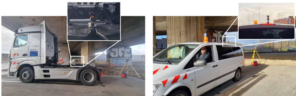
Figure 8: Load vehicles with 360° prisms for tracking with RTS, left: truck tractor, right: small van
