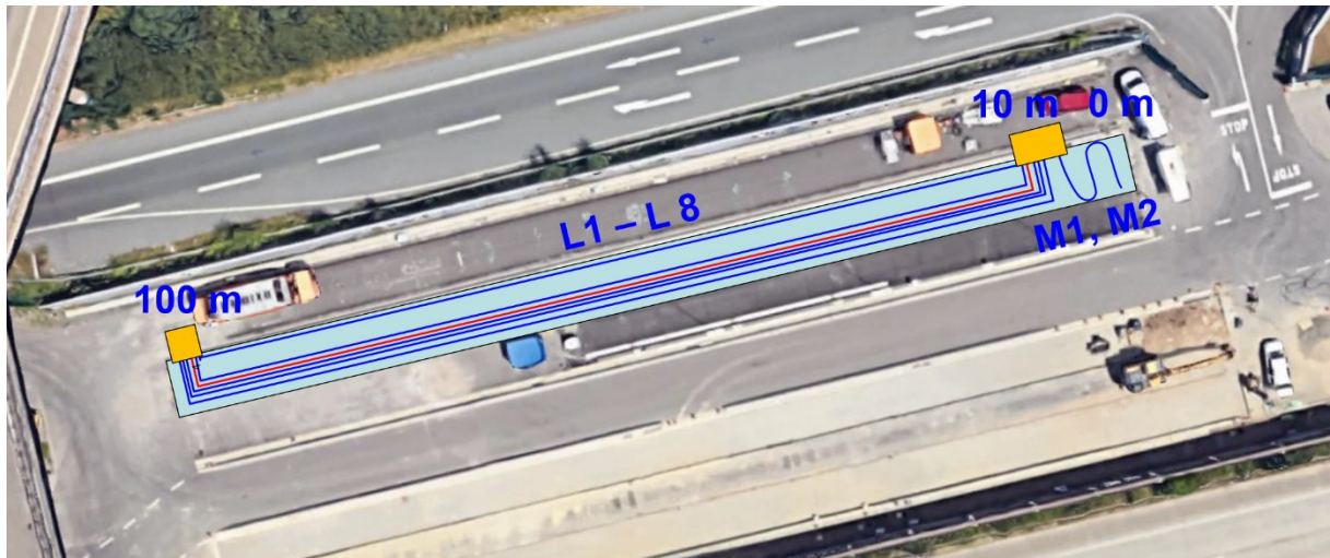
Figure 5: View of the installation in plan at duraBASt test area (blue = strain, red = temperature)
