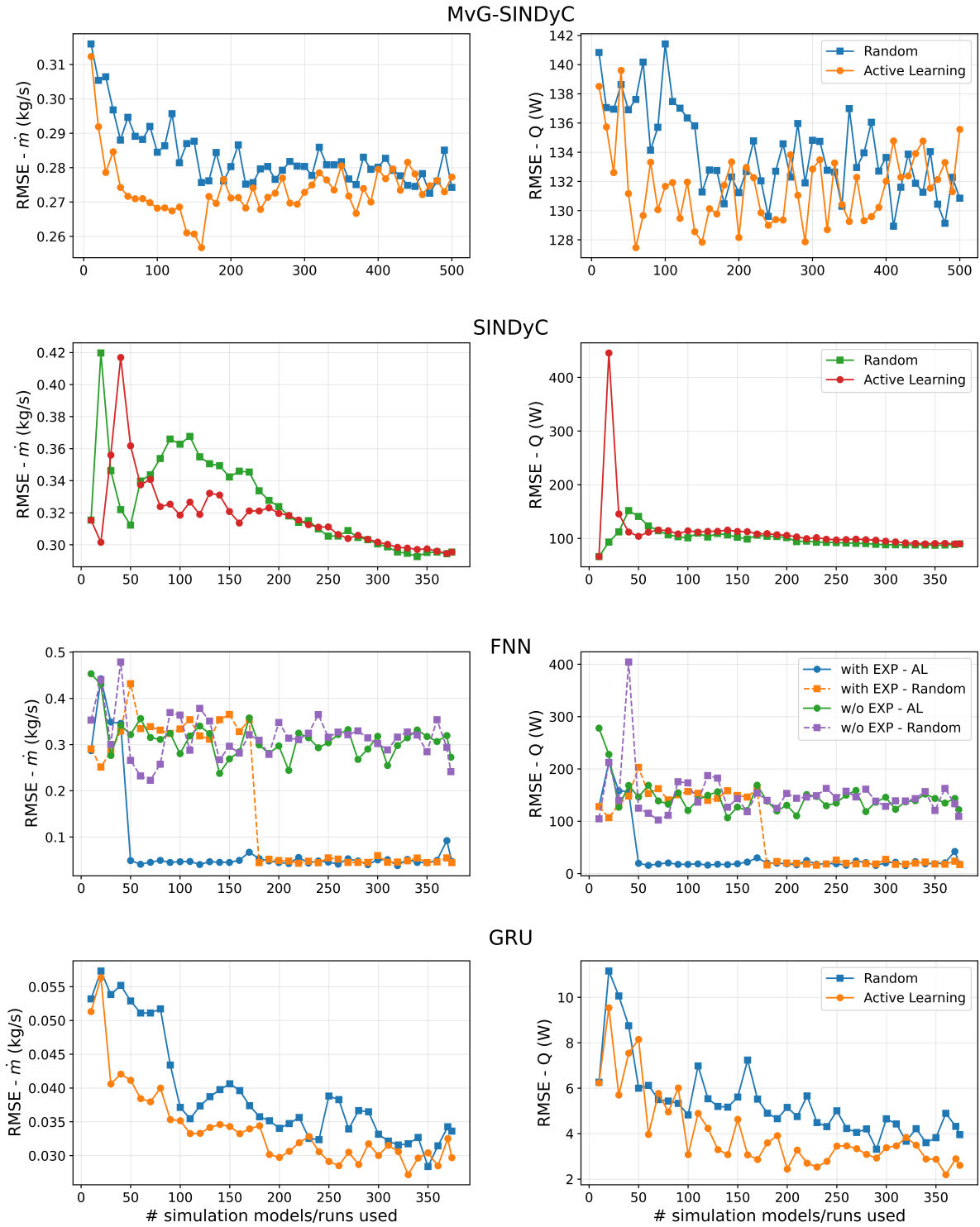
Figure 10: Prediction error trends (RMSE) pertaining to the mass-flow and power output for different models.
