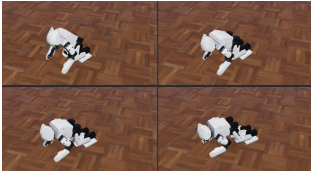
Fig. 4. Robot performing forward crawling motion in simulation.
