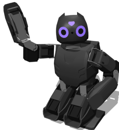
Fig. 1. DARwIn OP humanoid robot platform used in this study which was developed by Korean robot manufacturer Robotis
