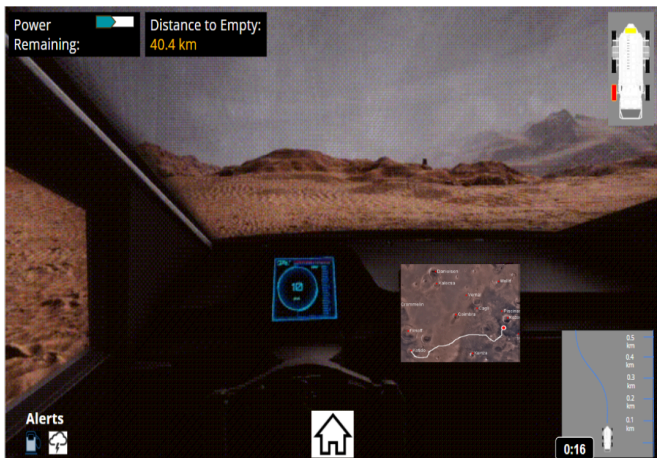
Figure 13. Flight/Driving display showing the rover trajectory map on the touchscreen beside the steering control, along with the forward Martian surface view.
