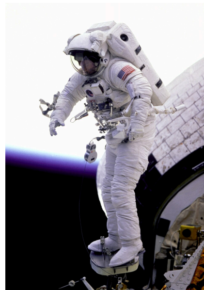
Figure 5. Astronaut performing an EVA while wearing the Space Shuttle spacesuit and attached to the EMU [7].
