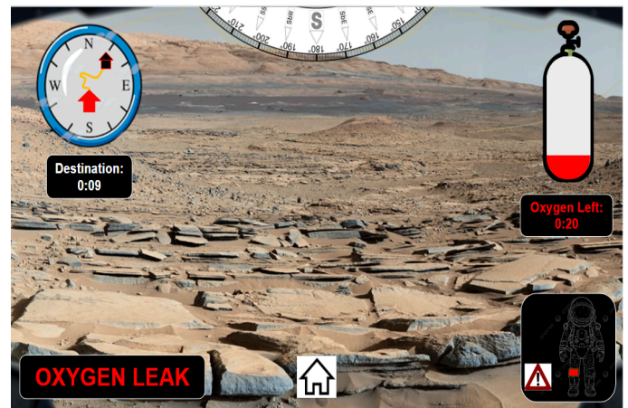
Figure 16. Emergency display depicting an oxygen leak in the spacesuit.
