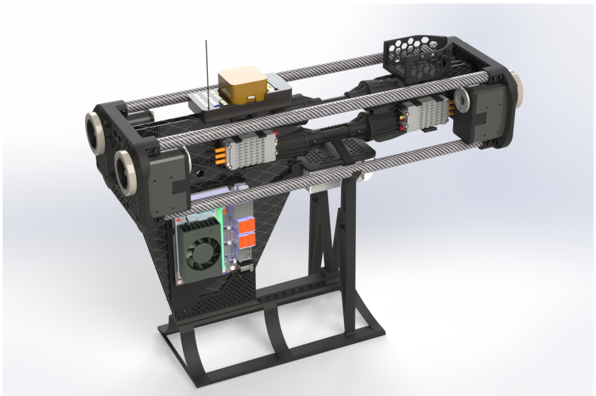
Figure 3.17: Shows the new assembled torso with electronics having Jetson Nano on one side and Voltage regulator and U2D2 board on the other.
